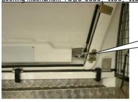
Check that latching works effortlessly and that the latch is well adjusted, adjust the lock or latch as required.
