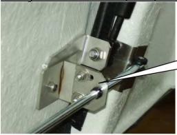
Check that the hatches are easy to close and the lock is well adjusted. Adjust the height as needed with the angle.
