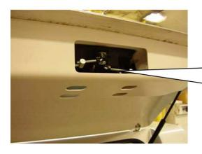
Middle lock can be adjusted by loosening the plastic latch and rotating the lock bar wound into a seam against the hook.
