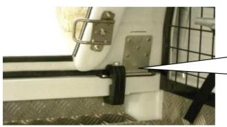
Do the same with the front fastener. NOTE! torsional moment 10 Nm at most.
