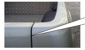
Clean first the truck bed side frame and place the transparent protective tape to truck bed side as well as the protective tape of rear wall.
