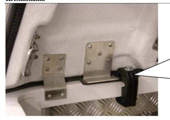
Pull the cap backwards on top of the vehicle so that it will not rub against the cabin in the front. Place the posterior fasteners to the place of installation as in the picture by pressing the cap from the outside towards the truck bed and simultaneously fastening the fasteners. NOTE! torsional moment 10 Nm at most.
