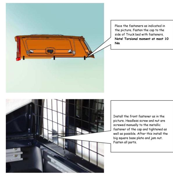
Locking mechanism: FMDC and FMEC
